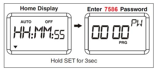
**Step4:** Below page with 1<sup>st</sup> digit blinking will appear **Press ENT** to stop blinking.
