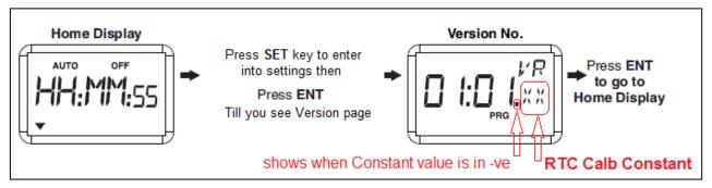
Step2: Verify range of existing "RTC Calibration Constant" is between 50 to 90.
